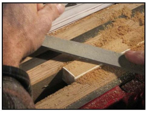
files to produce an edge which is perfectly flush to the wooden keystick. When done correctly, there will be no overhanging edge along the sides of the keys.
