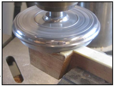
milling down process gives a completely flat surface on which to glue the new keytops.
